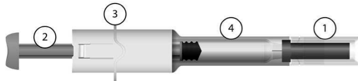
Picture 1. Syringe with an automatic needle protection system
