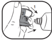
3. Using the key on the applicator cap to remove the star seal on the tube
